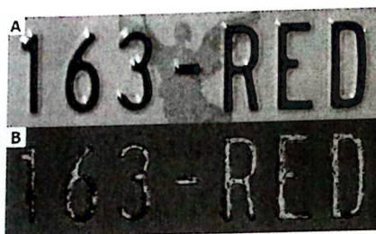
Fig. 4. This figure shows character segmentation. A) Original image B) Segmented image.
